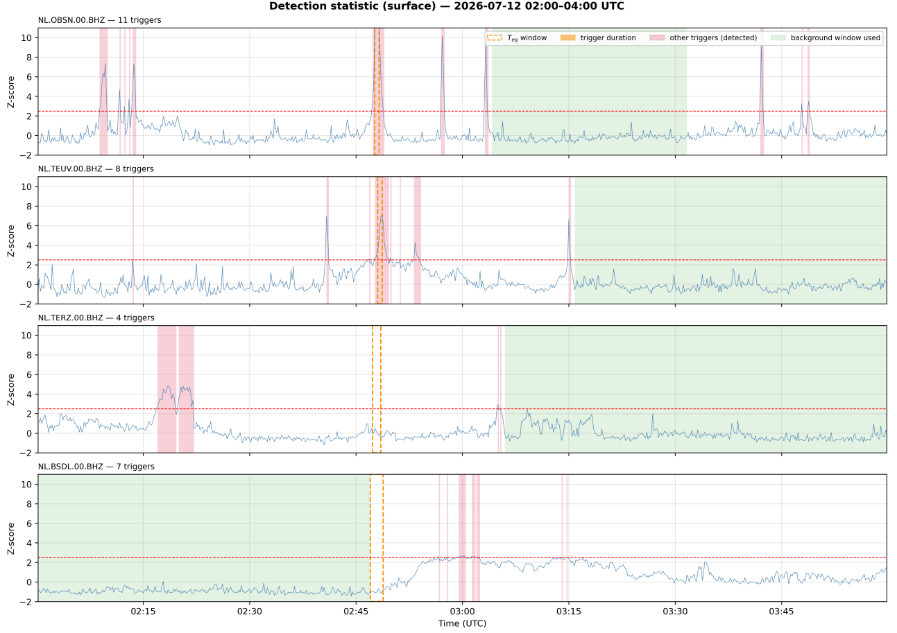
Figure 18: Detection statistic z(t) over the same chunk of Figure 6, for the borehole sensors (??) and for the co-located surface sensors (??). The dashed horizontal line is the detection threshold z_{\text{thresh}} = 2.5 ; the orange band is the trigger analyzed and the dashed orange lines delimit its T_{\text{eq}} window; the red bands are the other triggers of the same sensor, taken from the catalog for the borehole and detected locally for the surface; the green band is the background window actually used, i.e. the longest stretch in which neither sensor of the station has a trigger, with a guard of 60s. At TERZ and BSDL the surface statistic does not cross the threshold inside the T_{\text{eq}} window of the borehole, and the event is treated there as an upper limit.
