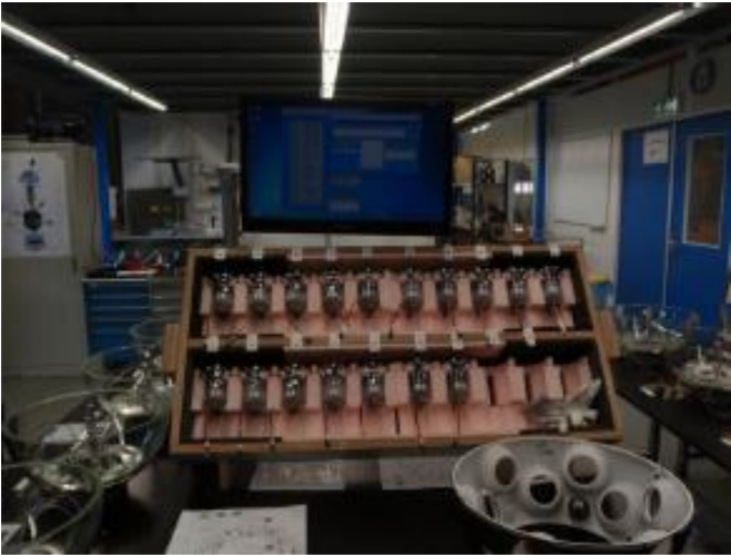
Inserting PMTs in structures
