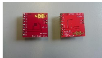
compass/accelerometer board (Paul T., Charles)
