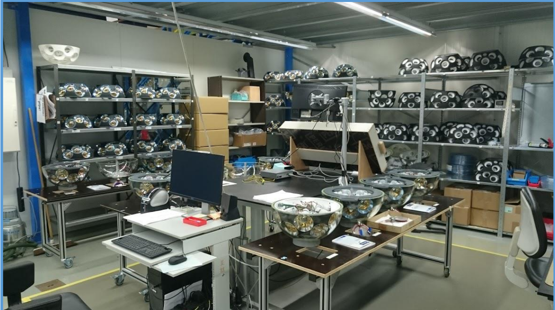
DOMs are assembled in halves and move around on tables
