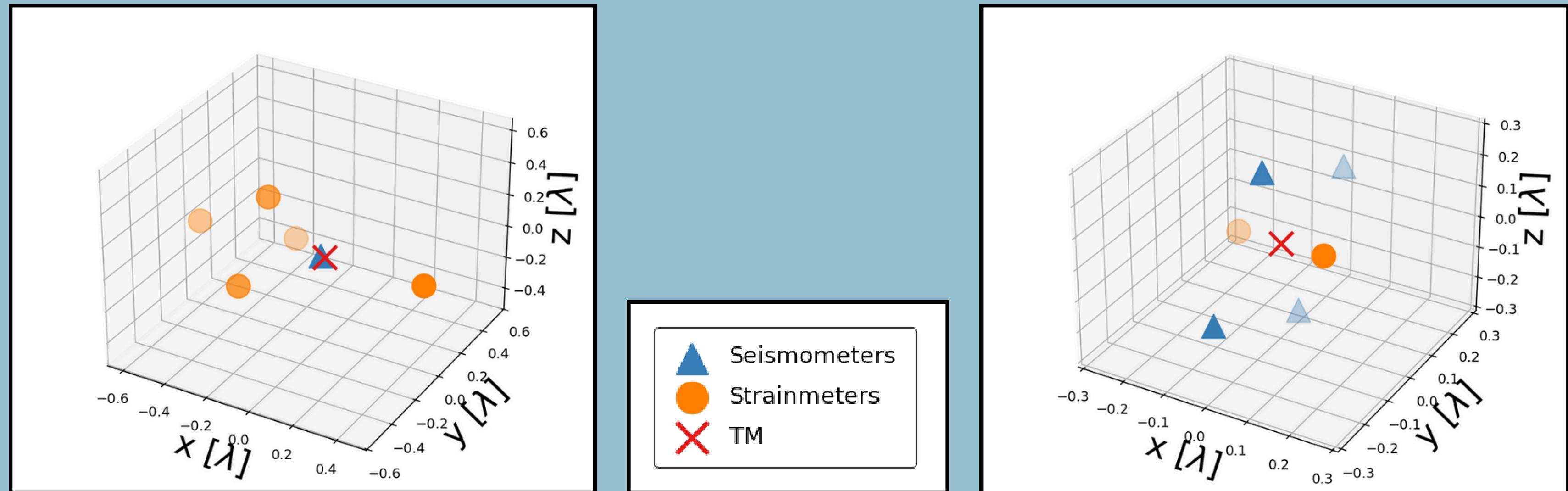
Resulting configurations optimising the positions of a sensor array which contains seismometers and strainmeters
