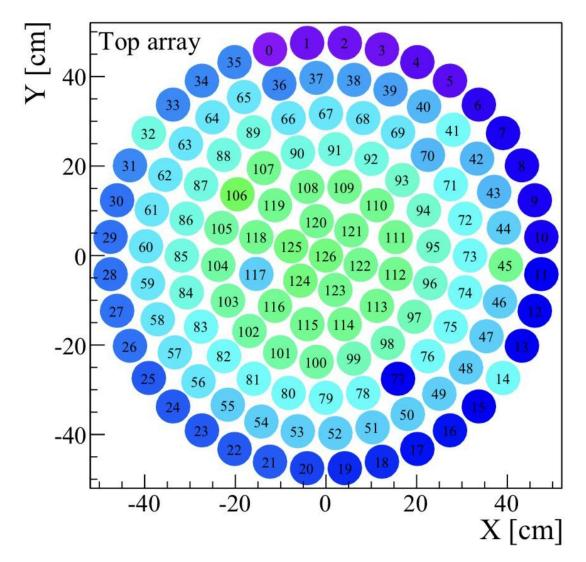
This figure shows the top PMT array in X–Y coordinates. Each circle is a PMT, and the color/size represents the amount of S2 light recorded.
