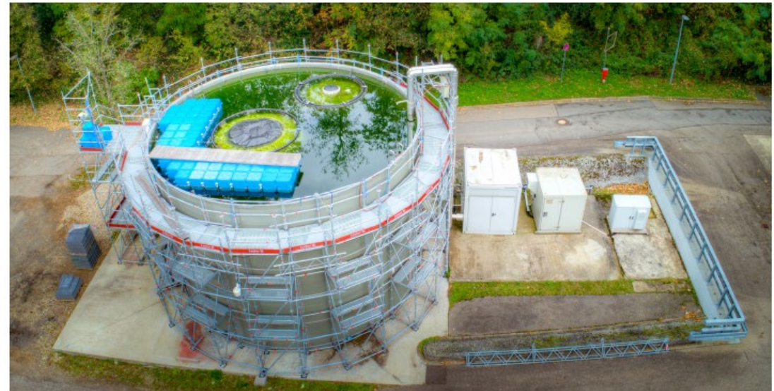
Figure 7: The test facility at MPIK: A 10 m diameter, 7 m height lake simulation tank, here with two bladders deployed. Next to the tank the water filtration system, and a small container for electronics and DAQ.
