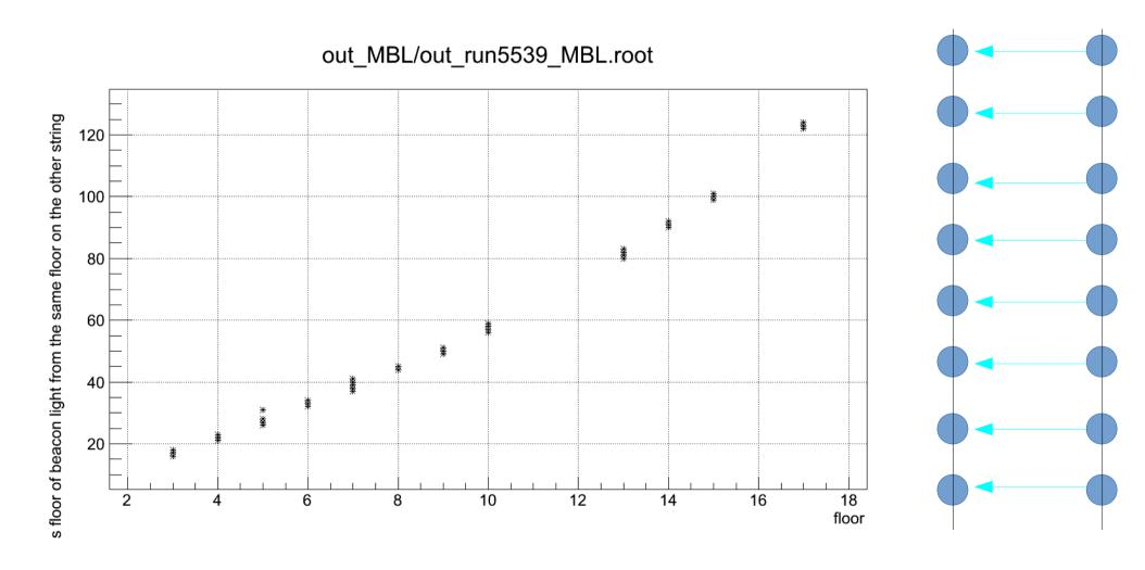
Change in horizontal light arrival times between high-luminosity run 5539 (March) and run 5080 (Jan) as a function of floor number.
