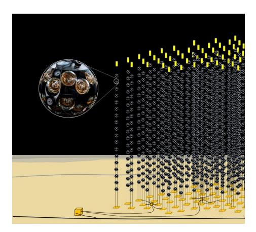
KM3NeT: Water Cherenkov detector on the bottom of the Mediterranean Sea
