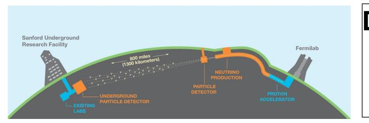
**DUNE:** Neutrino beam from Fermilab to detectors at 600m and 1300km distance Under construction, prototype detector at CERN
