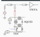
rf-SQUID multiplexing of TES/MMC microcalorimeter arrays for x-ray and gamma-ray spectroscopy.
