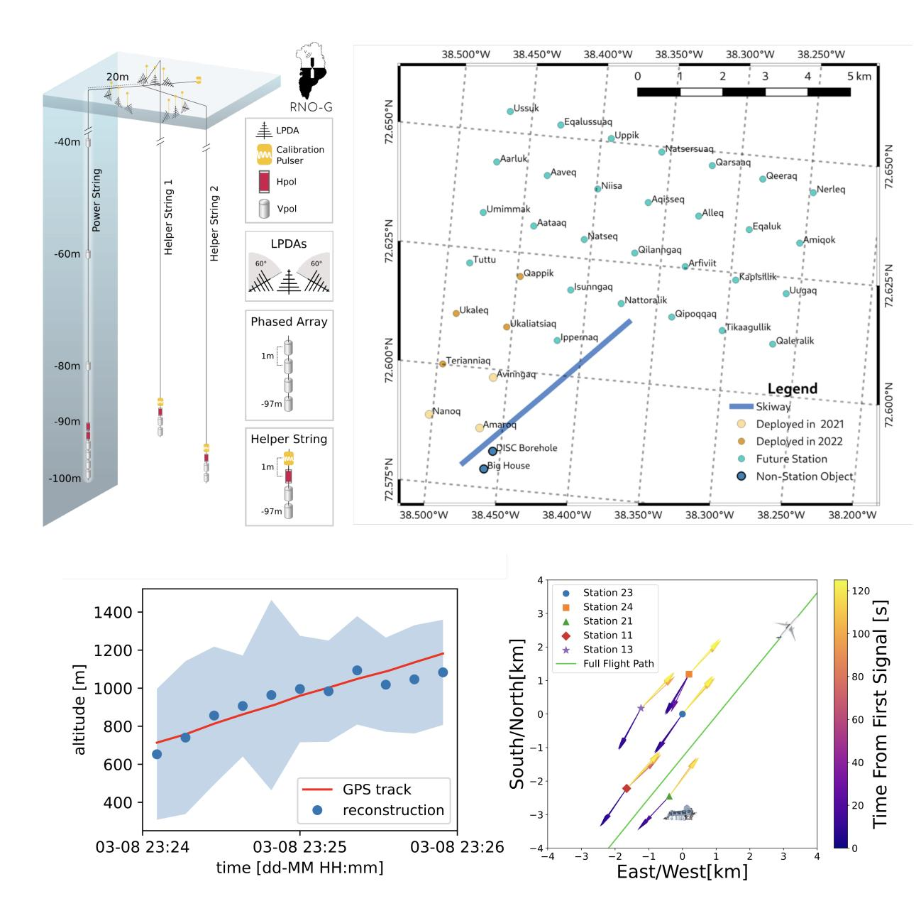
Figure 8: Left: the reconstruction of the local Radiosonde weather balloon, compared to the true reconstruction from the GPS file. Right: a set of reconstructed airplane events seen by five of the seven RNO-G stations. Jörg R. Hörandel - APP29, Soesterberg, 12-13 June 2025 24
