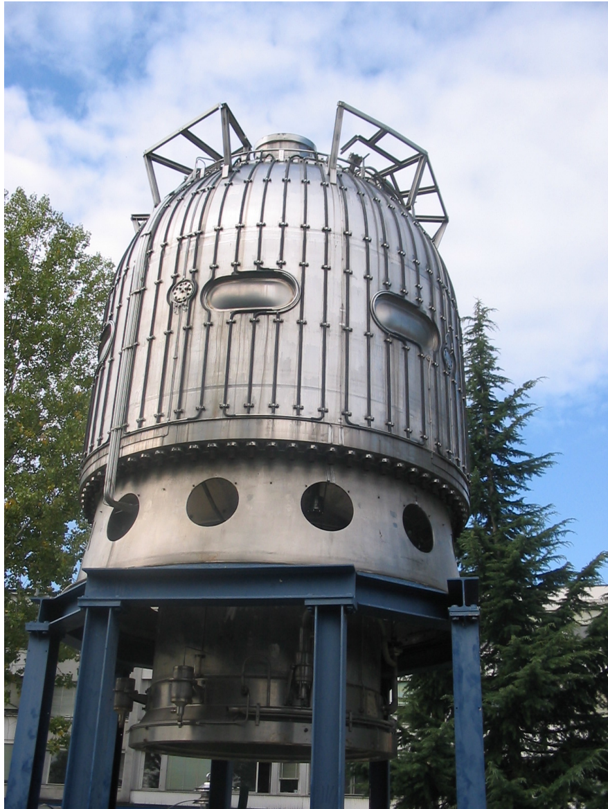
Big European bubble chamber at CERN (operation in 1970s) [1]
