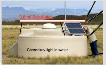
Water-Cherenkov detector and Scintillator have different response to electrons and muon
