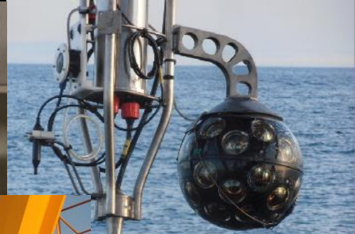
Little white structures prevent the HV bases and cables to touch each other
