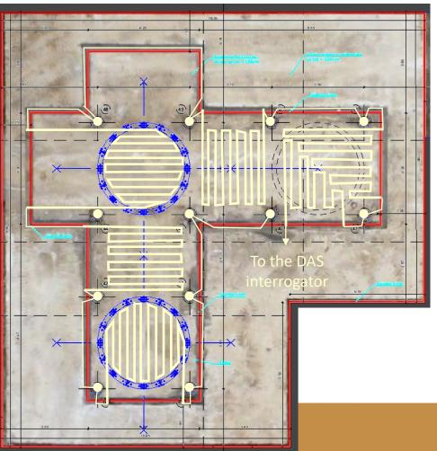
DAS systems allow in principle to measure strain variations along an optical fiber with space-time resolution ( $\Delta x \sim 1m$ ,  $\Delta t \sim 10 \mu s$ ).
