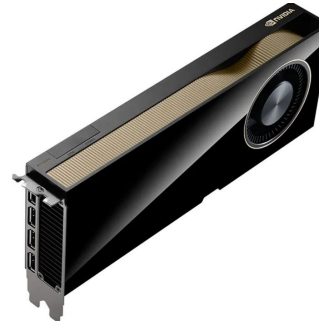
NVIDIA RTX 6000 18,176 cores 300W TDP
