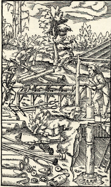
FIGURE 214—Agricola's simple suction-pump. On the left a man is hollowing out tree-trunks, for pipes, with augers (P, Q). 1556.
