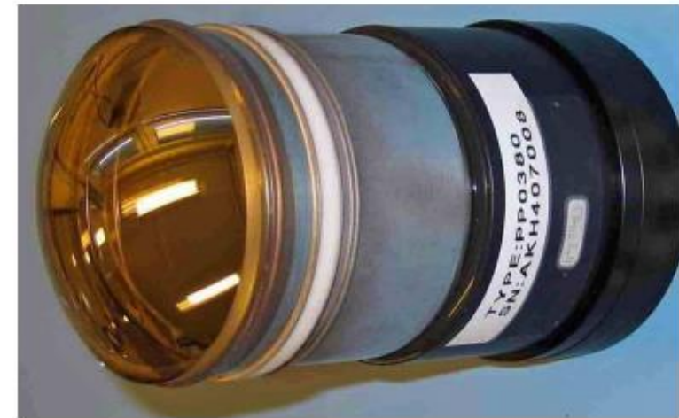
Figure 6.7: Left: a schematic and right: a photograph of the pixel-HPD.
