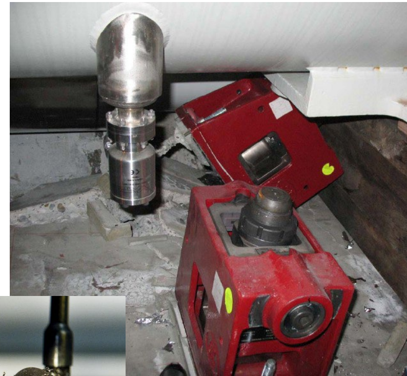
Top Right: LHC 2008 quench incident. Magnet anchors ripped out of concrete floor
