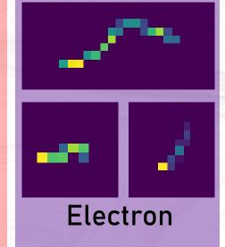
Natural radioactivity dataset acquired with Timepix4 bump-bonded to a 500 µm thick Silicon sensor.
