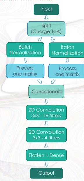
The network takes as input a 50x50x2 matrix, that is split into **two 50x50** matrices: **ToA + Charge**.
