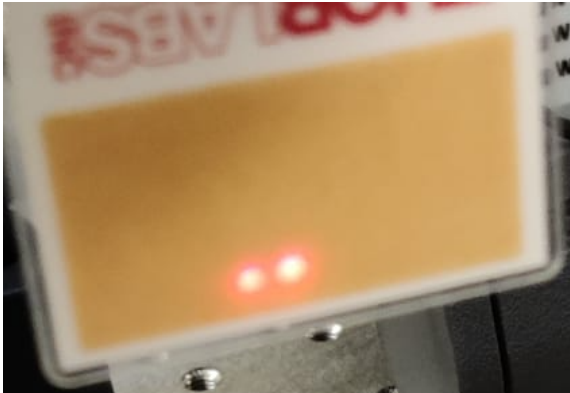
Figure 14: 0th and 1st order beams from 40MHz AOM.
