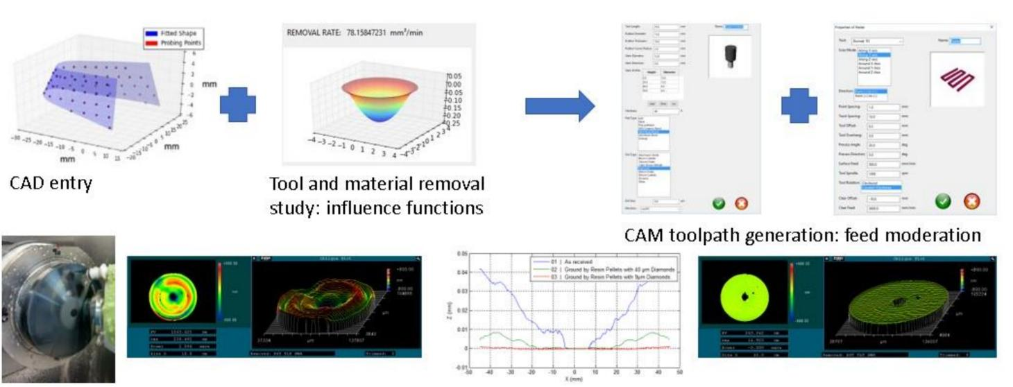
Corrective polishing with metrology feedback to CAM
