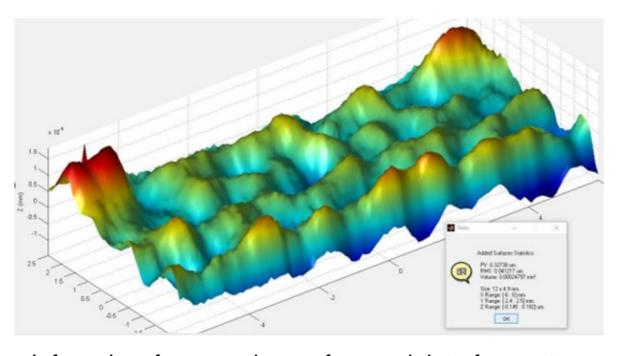
Inferred surface roughness from w..l. interferometry
