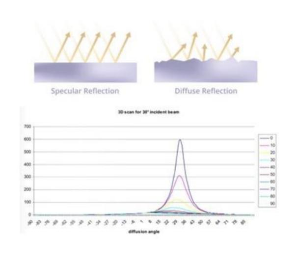
Measuring light scattering profile from silicon blanks on machined parts in transmission or reflection. For illumination white light source with a bank of filters is used. It is possible to measure scattering signal on reflection and transmission. Detection is conducted via detection of integrated flux or spectral analysis Easy calculation of BRDF and BTDF – Important for GW detector optics!
