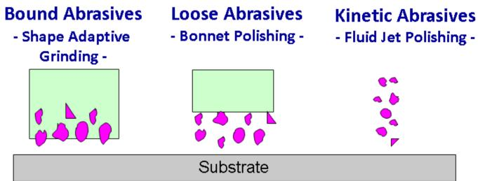
Schematic representation of different polishing
