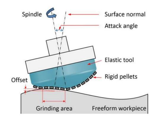
Different polishing methods and tools give specific surface roughness patterns. For freeform high precision optics as first step shape adaptive grinding is favourited and for polishing phase fluid jet polishing or Bonet polish are recommended.
