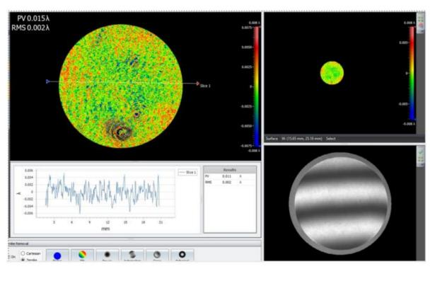
Interferogram from Zygo interferometer (top row), surface roughness (bottom left), white light interferogram (bottom right)
