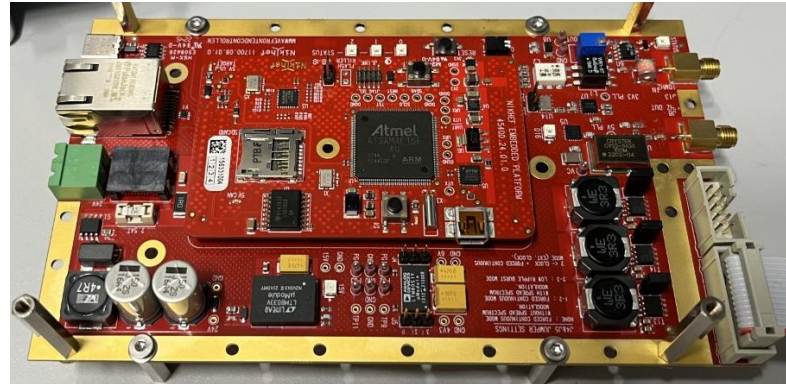
Front-end control board
