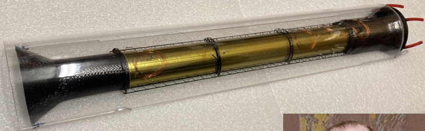
Layer 0 dummy with cooling concept
