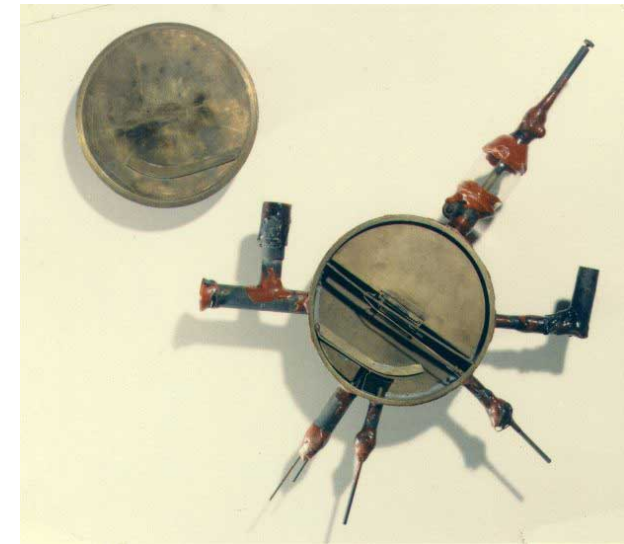
First Cyclotron(4.5 inches) Lawrence-Livingston (1933) 11 inch: accn. to 1 MeV.
