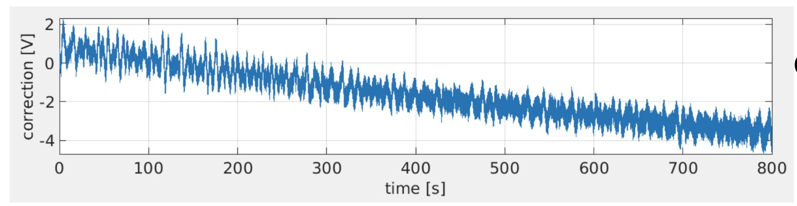
Longitudinal correction signal has been low passed and sent to the Inverted Pendulum
