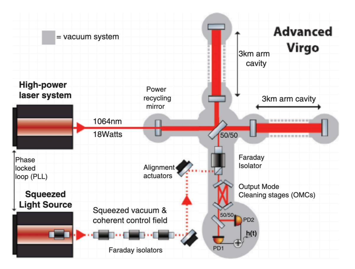
Frequency independent squeezing has been implemented for Virgo O3 run. In the lowfrequency region, we started to see the effect of the radiation pressure noise.
