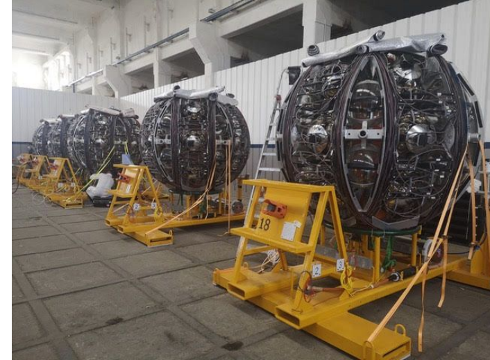
DUs installed on the Launching vehicle of Optical Module (LOM) before deployment (Yesterday, Malta)
