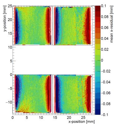
Uncorrected residuals from quad test beam
