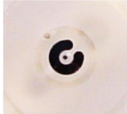
Mercury contact (Top view, seen through a glass plate)
