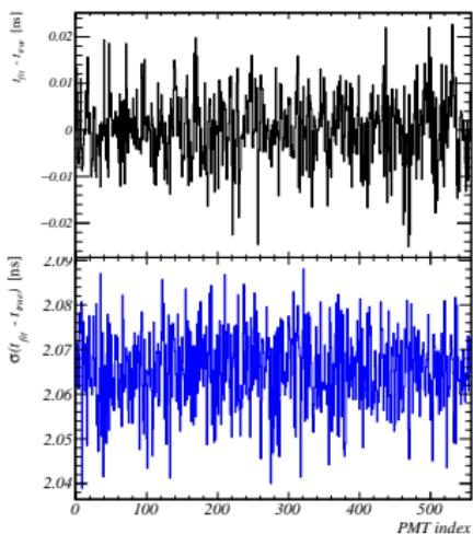
Stable PMT calibration after 15 minutes,  $\sim 2$  ns resolution
