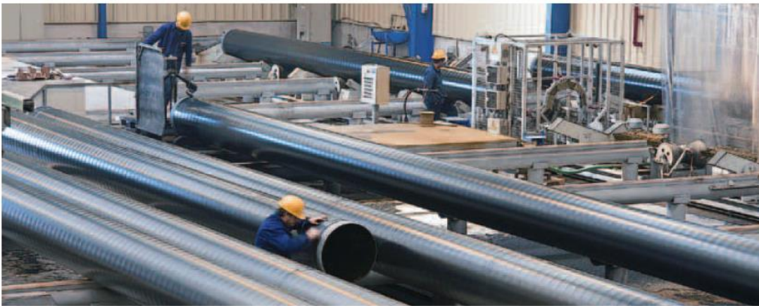
SAWH API 5L pipes being inspected during the coating operation.
