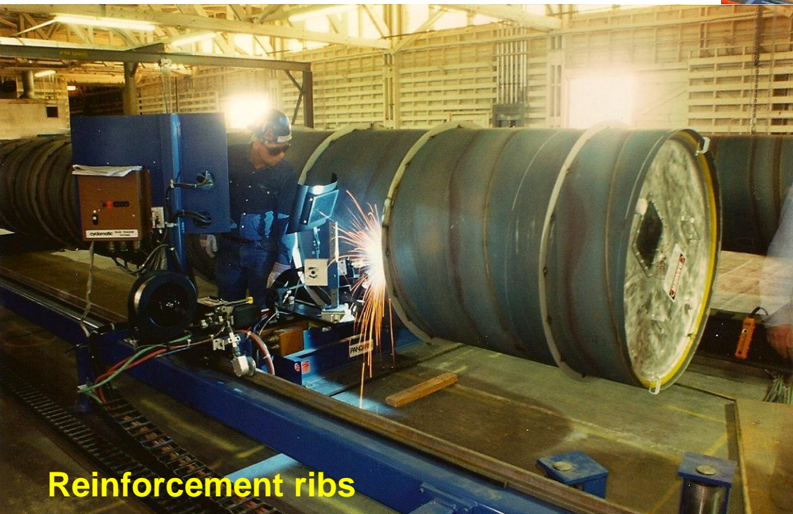
Spiral welding of beam tubes
