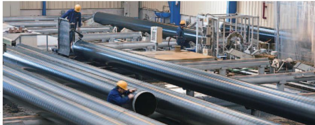
SAWH API 5L pipes being inspected during the coating operation.
