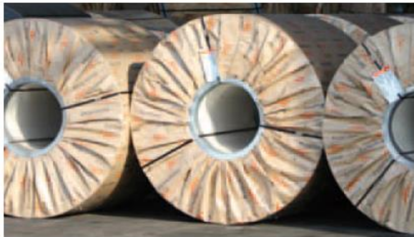
Pickled and oiled coils ready for overseas shipment (Fos-sur-Mer)
