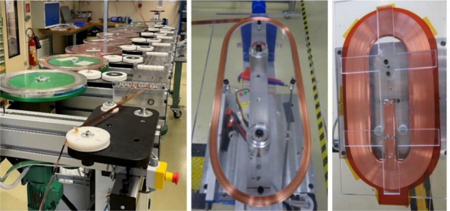
Demonstrator coil constructed for the HDMS project (funded CERN and ASI).
