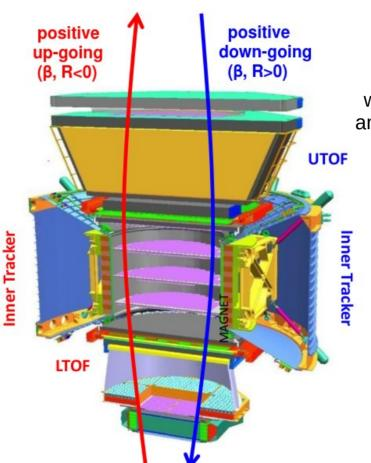
Charge identification, Z, with Inner Tracker ( $\Delta Z/Z\approx2\%$  for Z=6) and UTOF or LTOF ( $\Delta Z/Z\approx4\%$  for Z=6).
