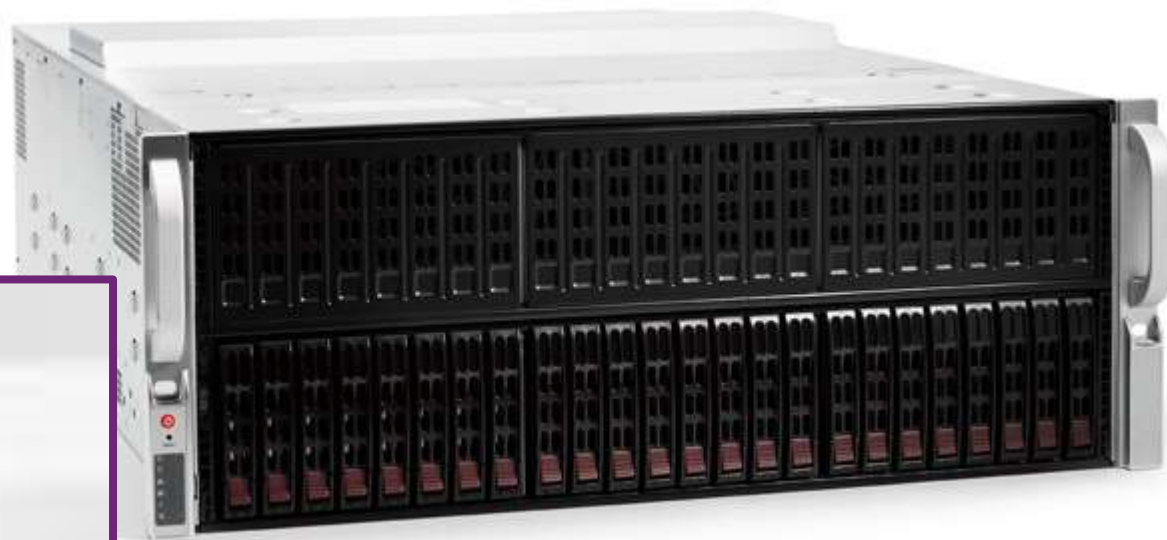
SuperMicro (branded as Lambda Blade) 4U chassis, supporting 10 consumer-grade GPUs ... ... with a bump
