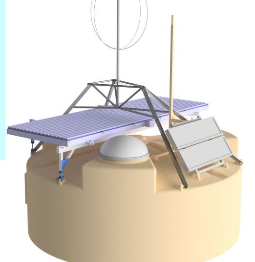
Shared infrastructure (solar power, battery, GPS timing, communications system) and integrated data acquisition
