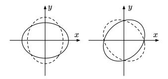
Gravitational waves can be detected by measuring these length changes
