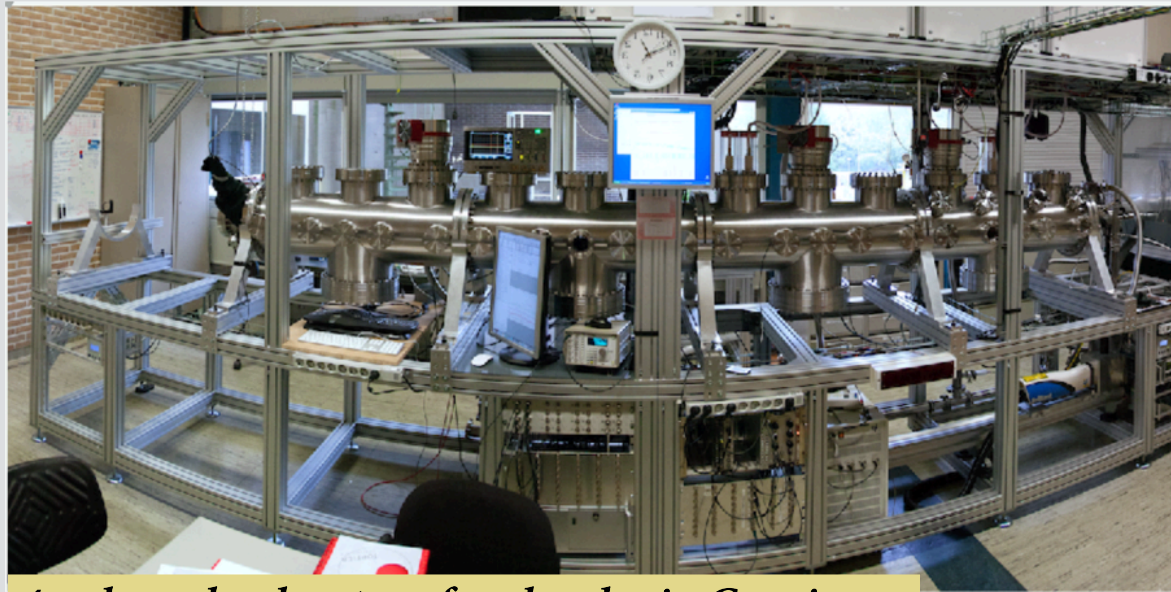
4 m long decelerator of molecules in Groningen
