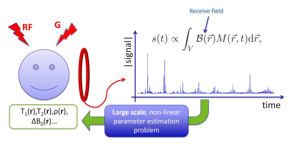
MR signal(t) = non-linear function(T1(r), T2(r), PD(r), scanner settings)
